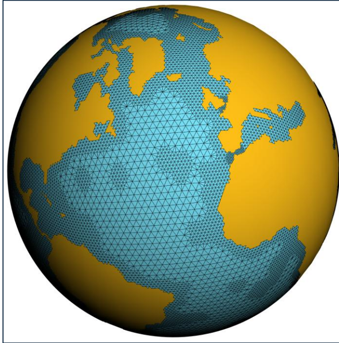
Computational mesh created with IMS 1.3 (Logemann & Klockmann 2025)
